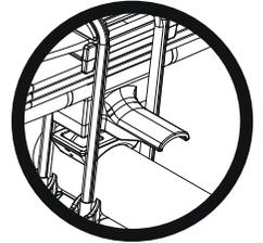
Fasten the air spring to the lower spring bracket.
