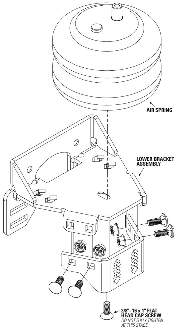
Fasten the air spring to the lower spring bracket.
