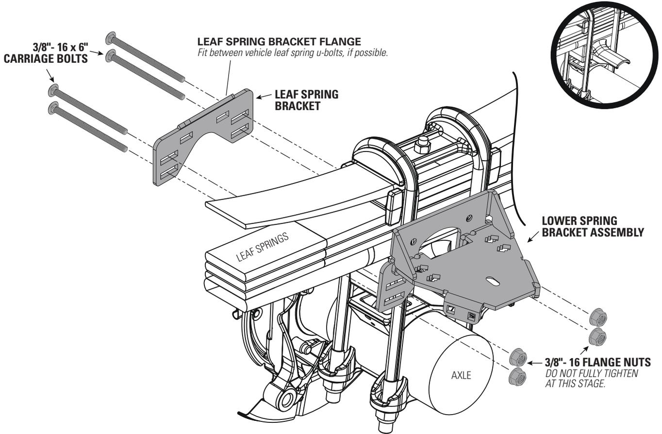
**1** Remove air spring and fastener from lower bracket assembly.
