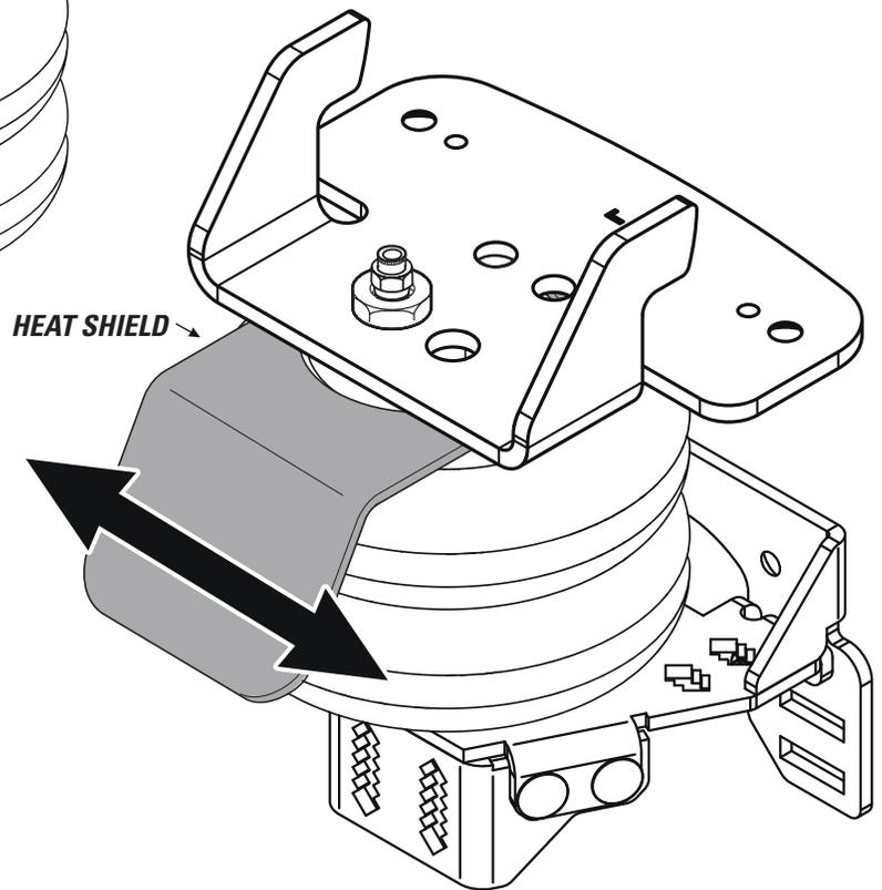
Position heat shield to closest point of exhaust. DO NOT PLACE DIRECTLY ABOVE AXLE.
