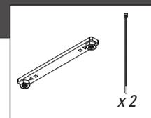
Attach nylon ties to the thread plate, as shown. These act as installation guides for the thread plate and upper bracket. They will be removed in a later step.
