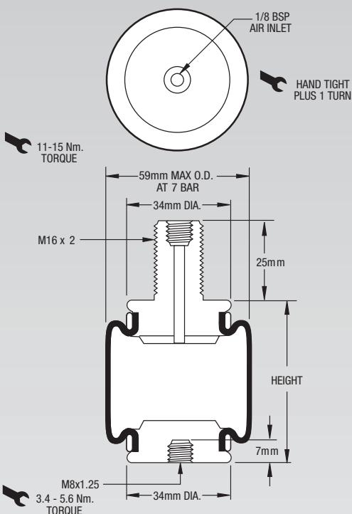
**NOTE:** This Airstroke actuator must be guided throughout the stroke.
