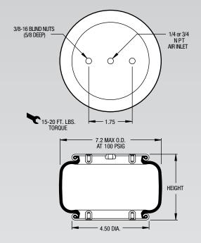
NOTE: The dotted line on the static data chart shows the force capabilities of the 160 when attaching an additional 0.5" pedestal, provided by the customer, to both ends of the air spring. If an additional pedestal is not used, the air spring will behave as the solid line depicts. Without the pedestal the rubber part will contact the mounting surface at the height of 2.9". This could cause wear prematurely to the rubber part.
